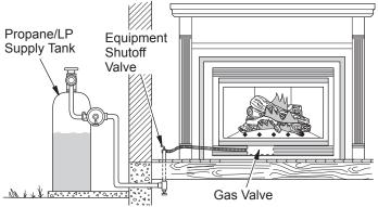
Figure 34 - Checking Gas Joints for Propane/LP Gas Fireplace
